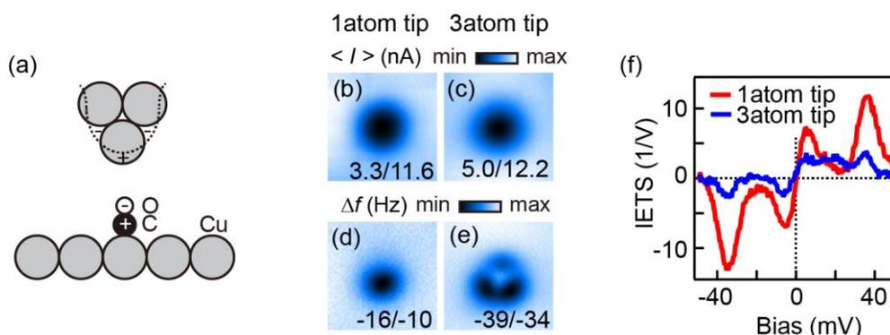
Fig.1 (a) Schematic image of dipole moments at the apex of the tip and the CO molecule. Constant-height, (b)[(c)] current and (d)[(e)] frequency shift images for a CO molecule on Cu(111) by a single-atom tip [three-atom tip]. (f) Normalized IETS for a CO molecule with a single-atom tip [three-atom tip].
